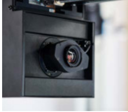
Camera system based on a CMOS sensor
