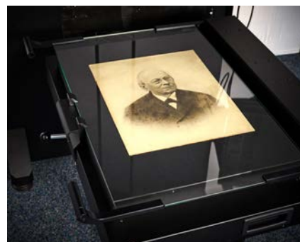
Photo table with glass plate and soft pad for very careful handling
