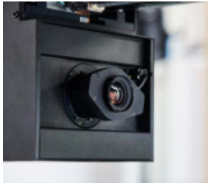
Camera system based on a CMOS sensor
