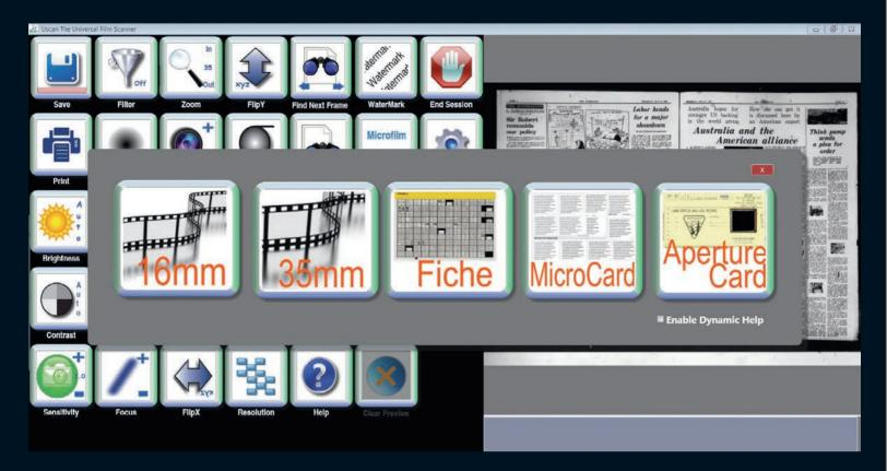
The touchscreen interface makes UScan operation easy for walk-up patrons, using system presets for different media. For advanced preservation scanning, the settings can be directed manually.
